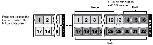
Each lit input button beyond input 1 indicates 3 percent of the total input volume is applied to the output. The flashing button indicates an additional 1.5 percent.
